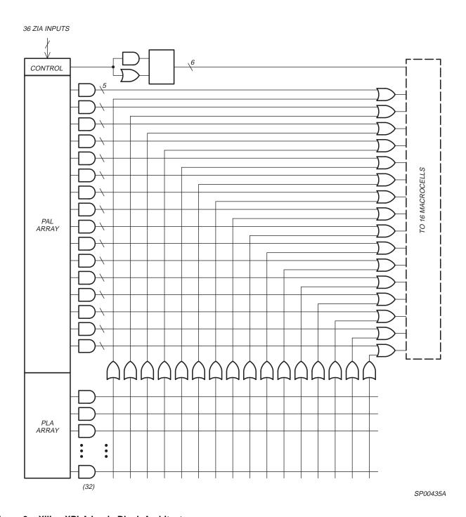
Figure 2: Xilinx XPLA Logic Block Architecture
