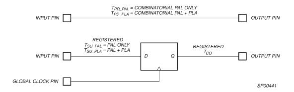
Figure 4: CoolRunner Timing Model
